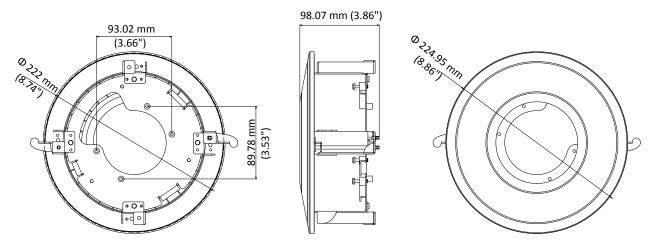
\*  $\Phi$  222 mm ( $\Phi$  8.86") is the diameter for the cable hole on the ceiling.
